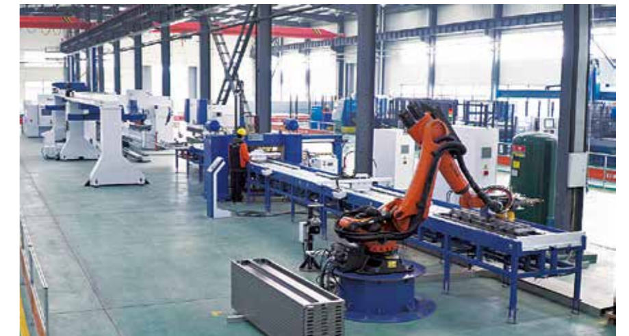
Automatic sheet metal processing system (Elevator industry)
