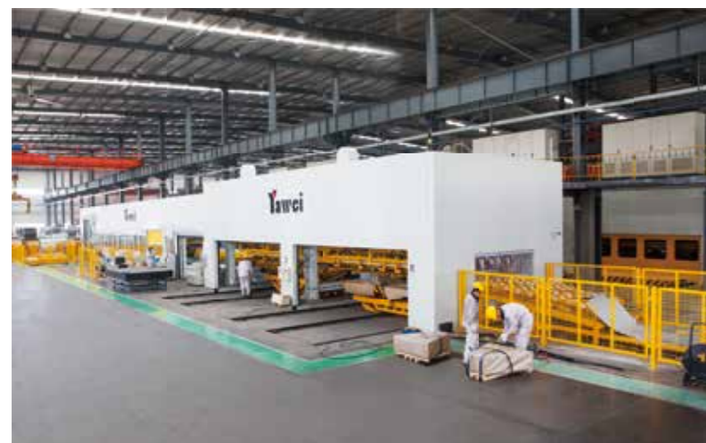
Cut to Length Line With Oscillating Shear
